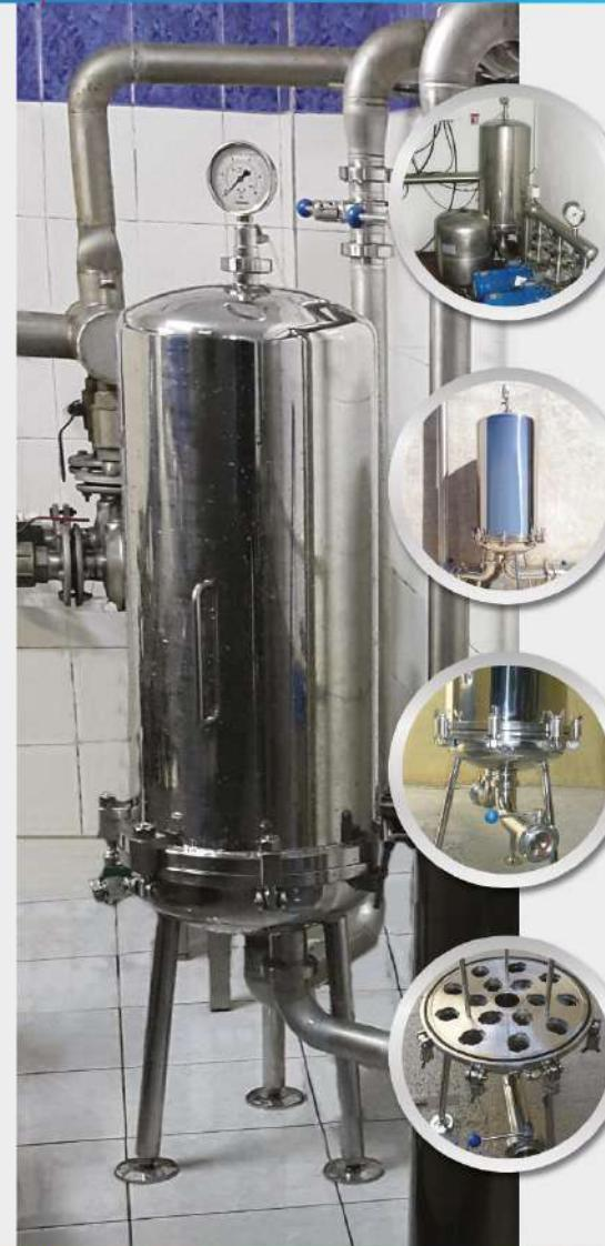
"Membrane" means "dice" in the Latin Alphabet. Membrane filters have determined diameter. They are absolute filters that do not allow to pass the largest diameter particles and microorganisms. The pressure-resistant membrane filter's pore size is in micron level. They have spongy porous structure. Membrane filters are produced with 0.1 -10 µm pore diameter ranges. Membrane filtration is a physical filtration.
